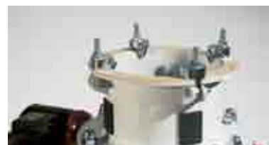
Silo flange with fixing blocks
