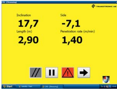
Main menu: Drilling angles, hole length and ROP Drill handling, alarm
