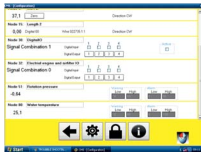
Trouble shooting menu: Transducer values, zero setting
