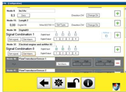
Configuration menu: Activation of transducers changing of direction, setting of transducer types
