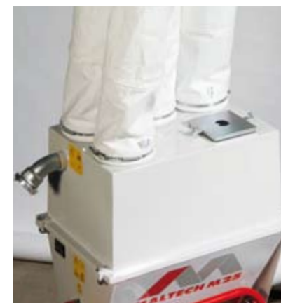
Feedhood for the conveyor system
